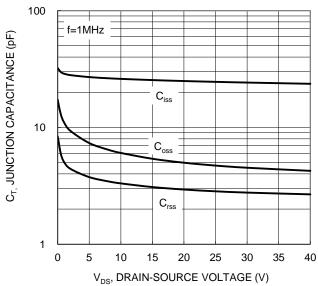
Figure 10. Typical Junction Capacitance
