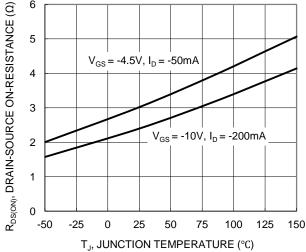
Figure 7. On-Resistance Variation with Temperature
