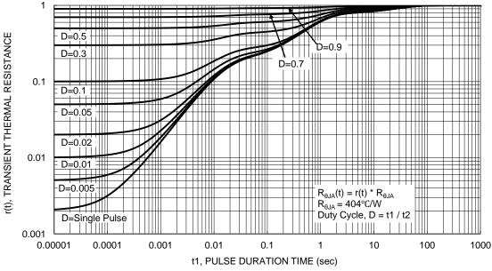
Figure 12. Transient Thermal Resistance
