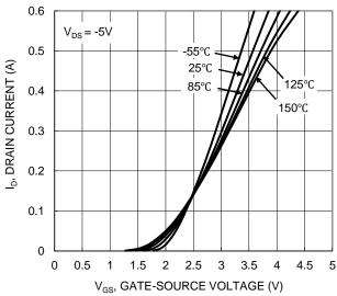
Figure 2. Typical Transfer Characteristic
