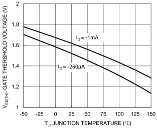
Figure 8. Gate Threshold Variation vs. Ambient Temperature
