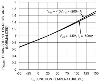
Figure 6. On-Resistance Variation with Temperature
