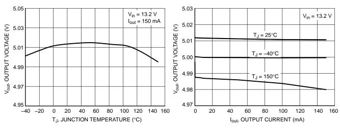
Figure 3. Output Voltage vs. Temperature
