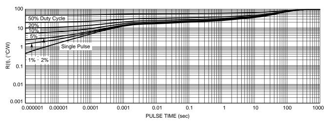
Figure 21. Transient Thermal Response (SOIC-8 Fused)
