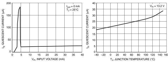
Figure 9. Quiescent Current vs. Input Voltage
