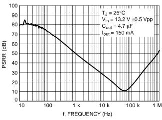
Figure 14. Ripple Rejection vs. Frequency
