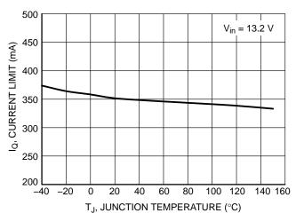
Figure 6. Current Limit vs. Temperature
