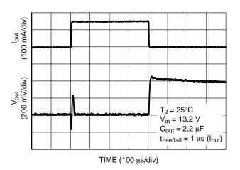
Figure 12. Load Transient
