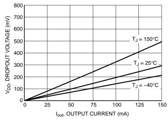
Figure 7. Dropout Voltage vs. Output Current
