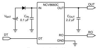
Figure 1. Application Diagram
