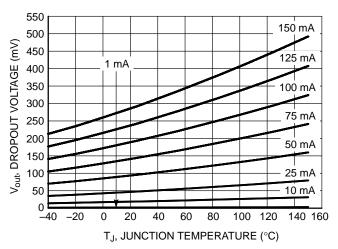
Figure 8. Dropout Voltage vs. Temperature
