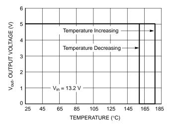
Figure 17. Thermal Shutdown vs. Temperature
