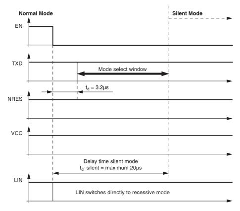
Figure 4-2. Switch to Silent Mode
