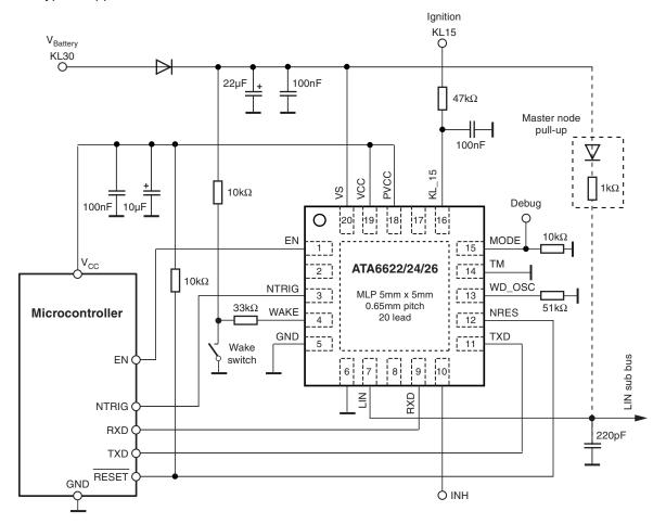
Figure 9-3. Application Circuit with External NPN-Transistor
