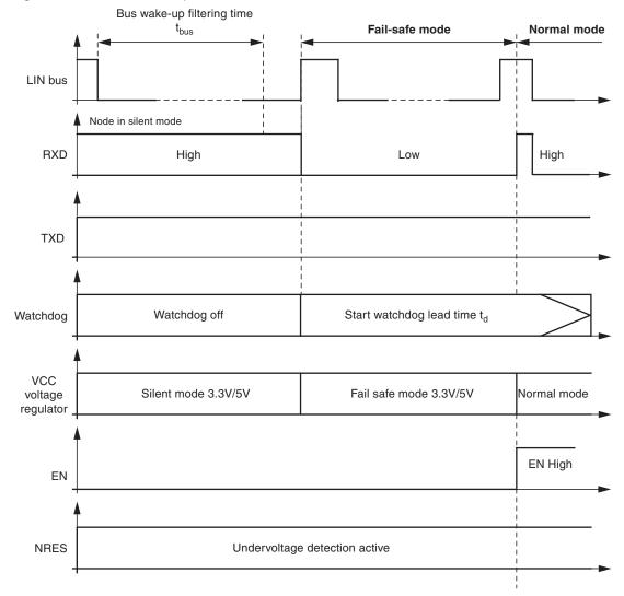
Figure 4-3. LIN Wake Up from Silent Mode
