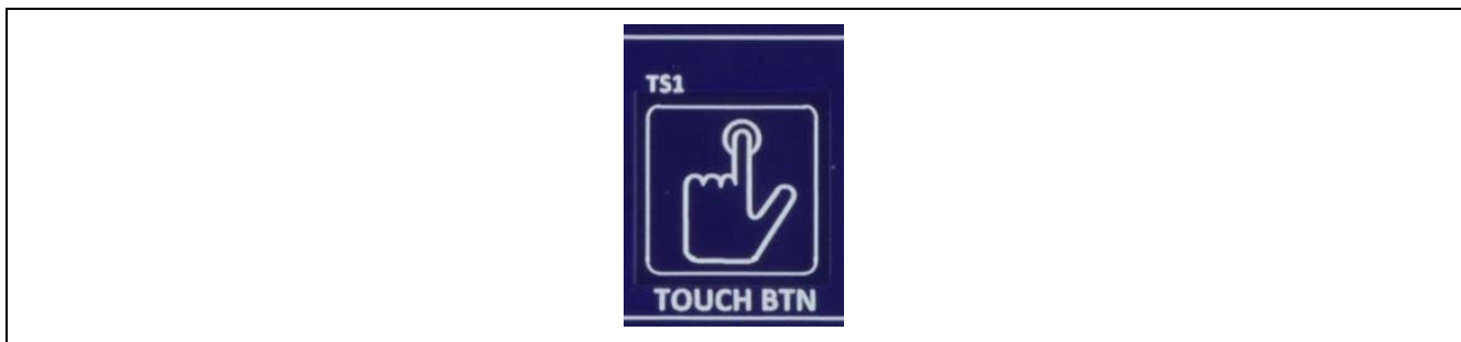
Figure 19 Capacitive touch button on target board (top)
