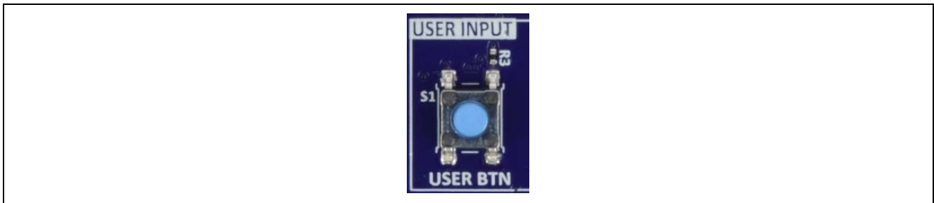
Figure 14 User switch (S1) on target board
