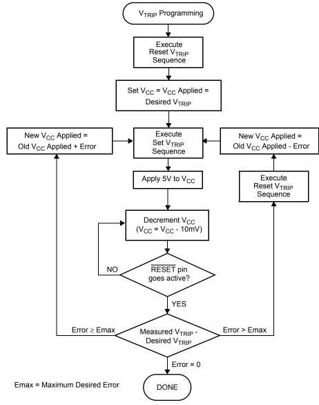
FIGURE 3.  $V_{\text{TRIP}}$  PROGRAMMING SEQUENCE FLOW CHART
