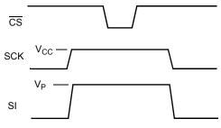
FIGURE 2. RESET VTRIP VOLTAGE
