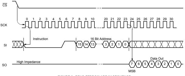
FIGURE 5. READ EEPROM ARRAY SEQUENCE
