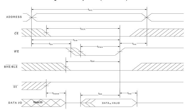
Figure 18. Write Cycle No. 3 (WE Controlled) <sup>[36, 37, 38]</sup>
