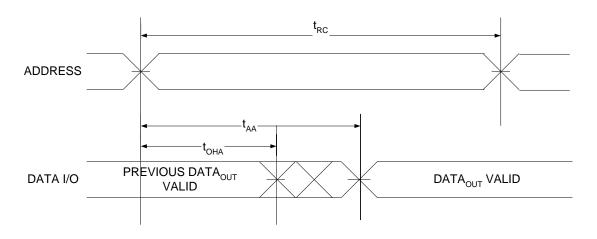
Figure 14. Read Cycle No. 2 of CY7C1061GE (Address Transition Controlled) <sup>[26, 27]</sup>
