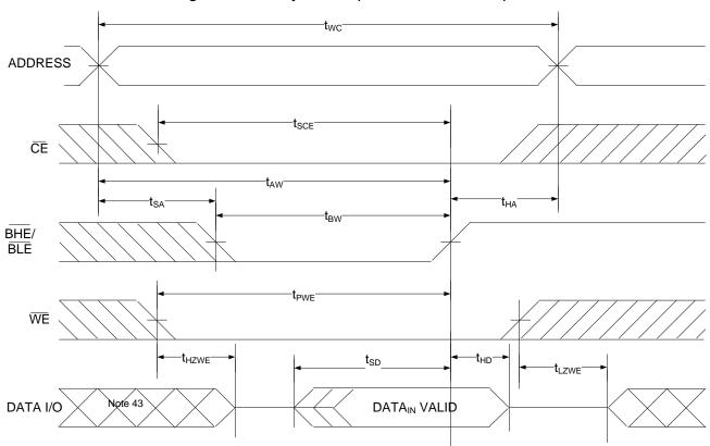
Figure 19. Write Cycle No. 4 ( $\overline{\text{BLE}}$  or  $\overline{\text{BHE}}$  Controlled) [40, 41, 42]
