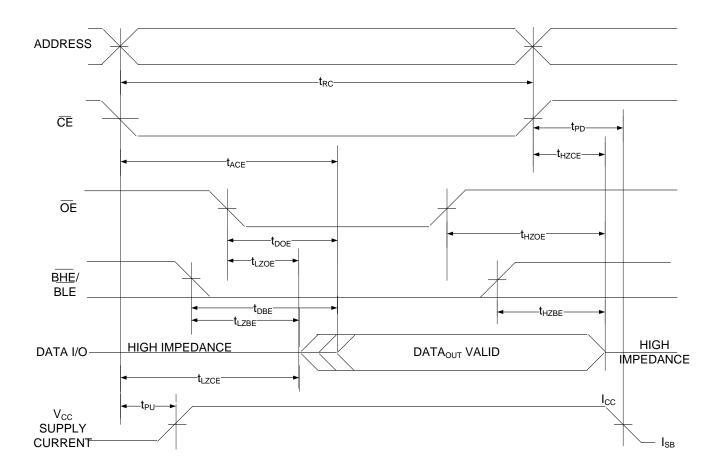
Figure 15. Read Cycle No. 3 (DE Controlled) <sup>[28, 29, 30]</sup>
