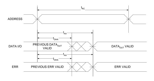
Notes 26. The device is continuously selected,  $\overline{OE} = V_{IL}$ ,  $\overline{CE} = V_{IL}$ ,  $\overline{BHE}$  or  $\overline{BLE}$  or both =  $V_{IL}$ . 27.  $\overline{WE}$  is HIGH for read cycle.
