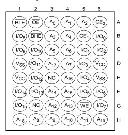
Figure 3. 48-ball VFBGA (6 × 8 × 1.0 mm) Pinout, Single Chip Enable without ERR, Address MSB A19 at Ball G2, CY7C1061G<sup>[3]</sup> Package/Grade ID: BV1XI
