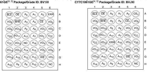
Figure 6. 48-ball VFBGA (6 × 8 × 1.0 mm) Pinout, Dual Chip Enable with ERR, Address MSB A19 at Ball H6, CY7C1061GE<sup>[4, 5]</sup> Package/Grade ID: BVXI
