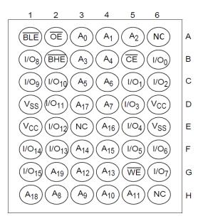
Note 3. NC pins are not connected internally to the die.
