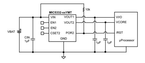
**Camera DSP Power Supply Circuit**
