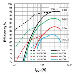
Figure 22: XR76205 efficiency, V<sub>IN</sub>=24V
