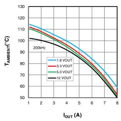
Figure 26: XR76208, V<sub>IN</sub>=24V
