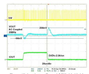
Figure 17: Load step, Forced CCM, 0A-4A-0A
