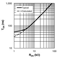
Figure 3:  $T_{ON}$  versus  $R_{ON}$
