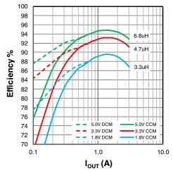
Figure 23: XR76203 efficiency, V<sub>IN</sub>=12V
