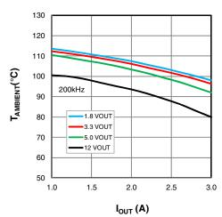
Figure 30: XR76203, V<sub>IN</sub>=24V
