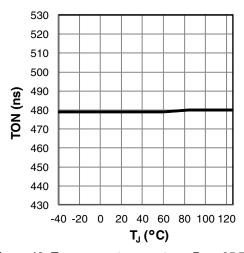
Figure 12:  $\text{T}_{\text{ON}}$  versus temperature,  $\text{R}_{\text{ON}}\text{=}35.7\text{k}\Omega$
