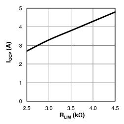
Figure 9: XR76203  $I_{OCP}$  versus  $R_{LIM}$
