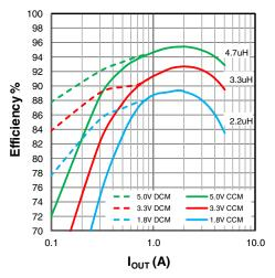
Figure 21: XR76205 efficiency, V<sub>IN</sub>=12V
