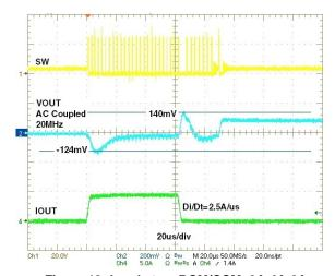
Figure 18: Load step, DCM/CCM, 0A-4A-0A
