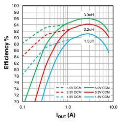
Figure 19: XR76208 efficiency, V<sub>IN</sub>=12V
