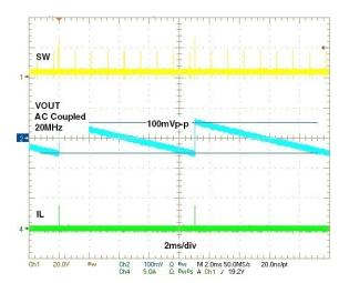
Figure 14: Steady state, DCM, I<sub>OUT</sub>=0A
