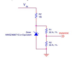
Figure 31: Selecting Forced CCM by deriving EN/MODE from  $V_{\rm IN}$
