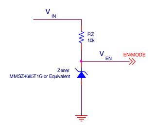
Figure 32: Selecting DCM/CCM by deriving EN/MODE from  $\rm V_{IN}$
