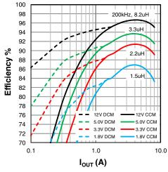
Figure 20: XR76208 efficiency, V<sub>IN</sub>=24V
