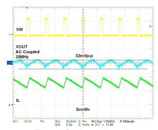
Figure 13: Steady state, I<sub>OUT</sub>=8A
