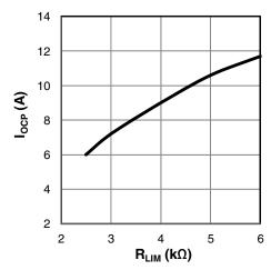
Figure 7: XR76208 I<sub>OCP</sub> versus R<sub>LIM</sub>
