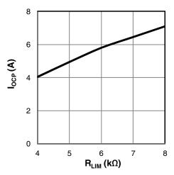
Figure 8: XR76205  $I_{OCP}$  versus  $R_{LIM}$
