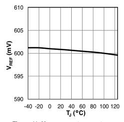
Figure 11: V<sub>REF</sub> versus temperature
