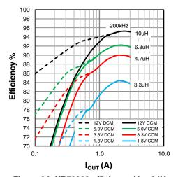
Figure 24: XR76203 efficiency, V<sub>IN</sub>=24V
