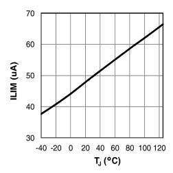
Figure 10: I<sub>LIM</sub> versus temperature
