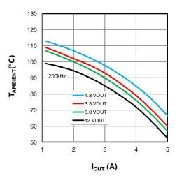
Figure 28: XR76205, V<sub>IN</sub>=24V
