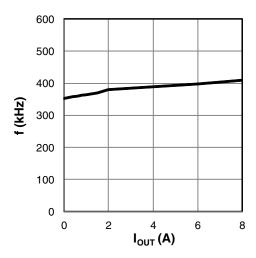
Figure 5: frequency versus I<sub>OUT</sub>
