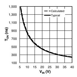
Figure 4: T<sub>ON</sub> versus V<sub>IN</sub>, R<sub>ON</sub>=27.4k
