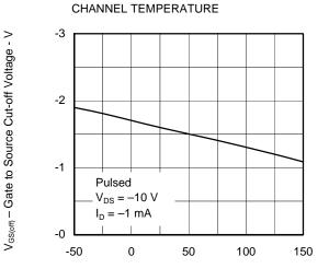
GATE TO SOURCE CUT-OFF VOLTAGE vs.
