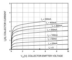
Figure 1. Static Characteristic
