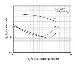
Figure 4. Turn On, Storage and Fall Time vs. Collector Current
