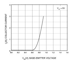
Figure 5. Base-Emitter On Voltage
