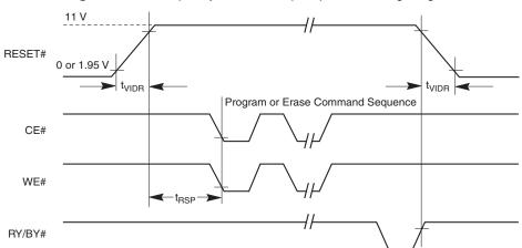
Figure 18.10 Temporary Sector Group Unprotect/Timing Diagram
