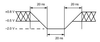
Figure 14.2 Maximum Positive Overshoot Waveform
