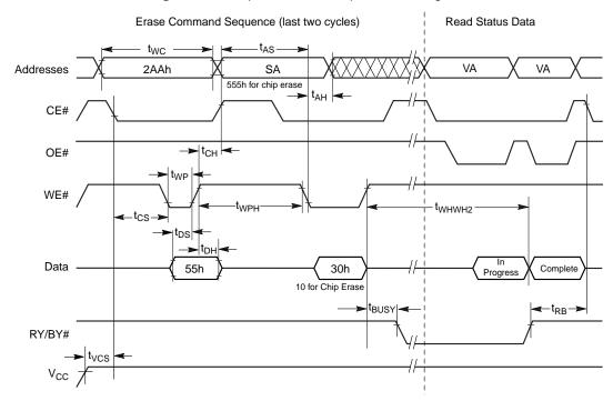
Figure 18.6 Chip/Sector Erase Operation Timings
