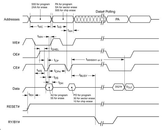
Figure 18.12 Alternate CE# Controlled Write Operation Timings
