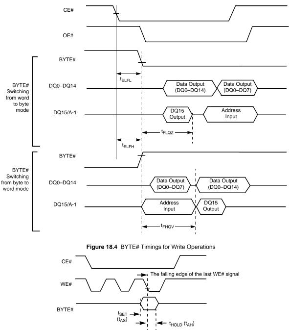
Figure 18.3 BYTE# Timings for Read Operations
