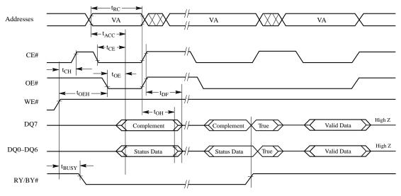
Figure 18.7 Data# Polling Timings (During Embedded Algorithms)
