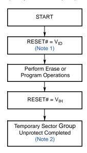
Figure 7.2 Temporary Sector Group Unprotect Operation
