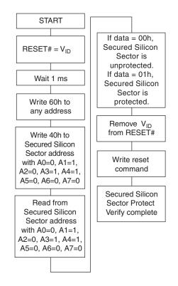
Figure 8.1 Secured Silicon Sector Protect Verify
