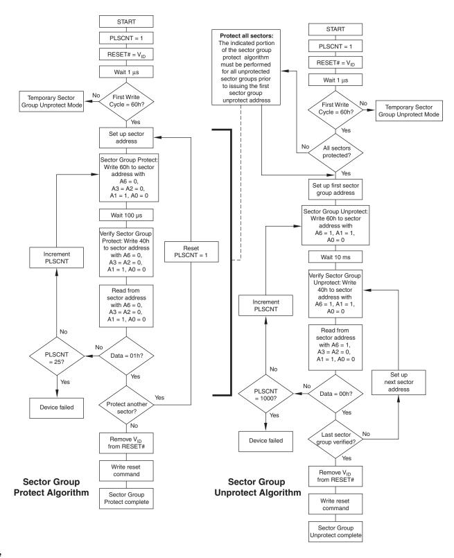
Figure 7.1 In-System Sector Group Protect/Unprotect Algorithms
