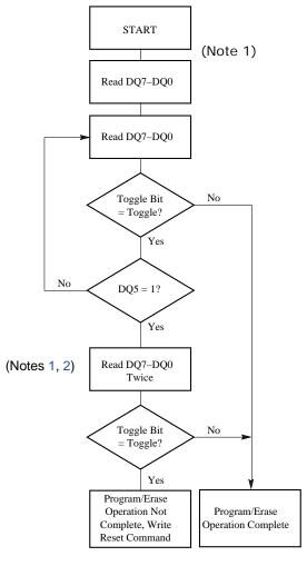
Figure 12.2 Toggle Bit Algorithm
