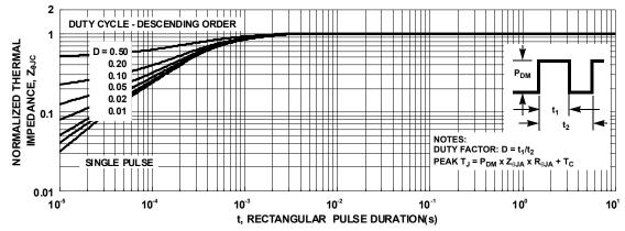
Figure 3. Normalized Maximum Transient Thermal Impedance
