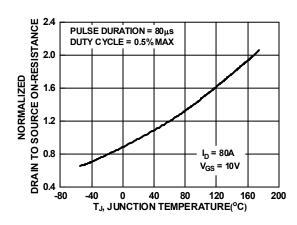
Figure 12. Normalized R<sub>DSON</sub> vs. Junction Temperature
