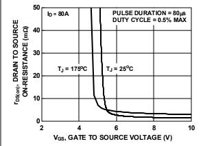
Figure 11. R<sub>DSON</sub> vs. Gate Voltage
