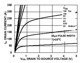
Figure 9. Saturation Characteristics
