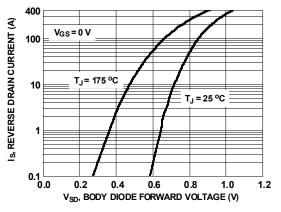
Figure 8. Forward Diode Characteristics
