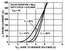
Figure 7. Transfer Characteristics
