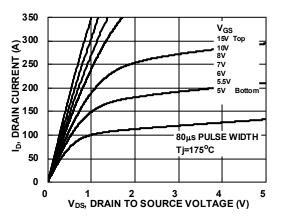
Figure 10. Saturation Characteristics
