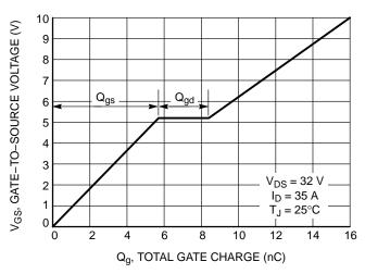
Figure 8. Gate-to-Source Voltage vs. Total Charge
