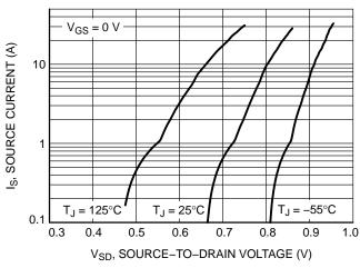
Figure 10. Diode Forward Voltage vs. Current
