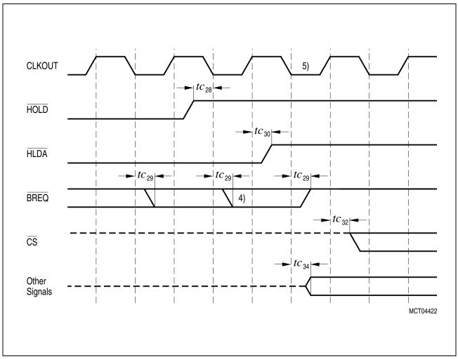
Figure 22 External Bus Arbitration, Regaining the Bus
