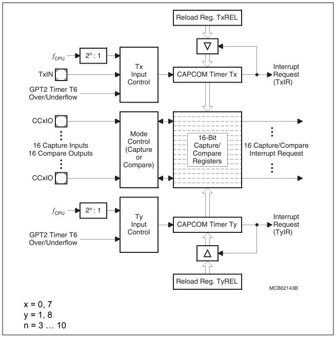
Figure 6 CAPCOM Unit Block Diagram
