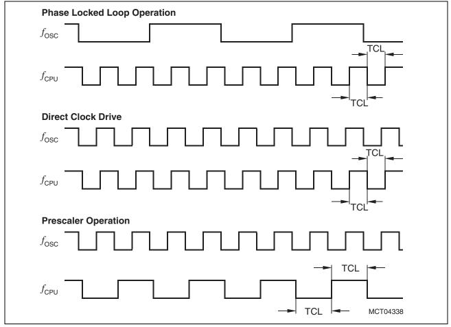
Figure 10 Generation Mechanisms for the CPU Clock
