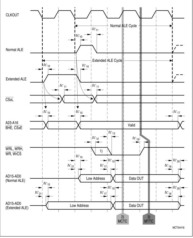
Figure 18 Multiplexed Bus, Write Access
