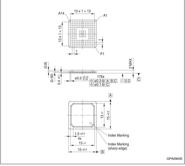
Figure 25 P-BGA-176-2 (Plastic Ball Grid Array Package)
