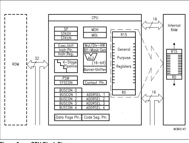
Figure 5 CPU Block Diagram
