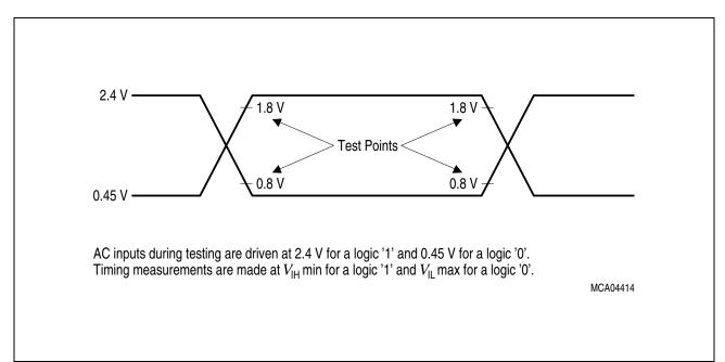
Figure 13 Input Output Waveforms
