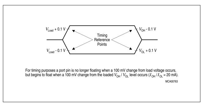
Figure 14 Float Waveforms
