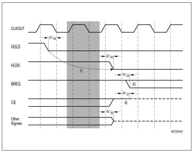
Figure 21 External Bus Arbitration, Releasing the Bus
