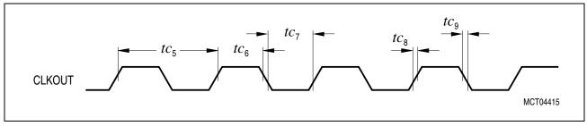
Figure 15 CLKOUT Signal Timing
