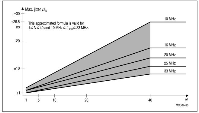
Figure 11 Approximated Maximum Accumulated PLL Jitter
