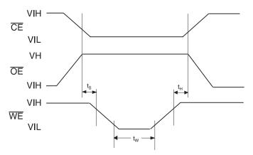
$t_S = t_H = 5 \mu s \text{ (min.)}$   $t_W = 10 \text{ ms (min.)}$  $V_H = 12.0 \text{ V} \pm 0.5 \text{ V}$
