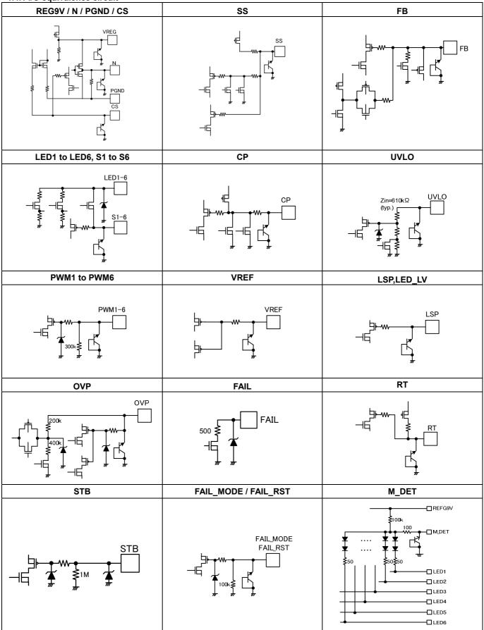
Figure 5. I/O equivalence circuit
