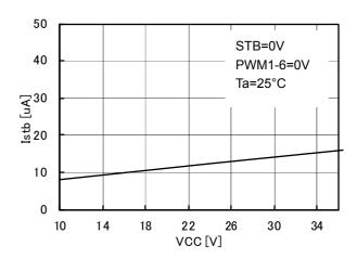
Figure 7. Stand-by circuit current
