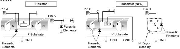
Figure 31. Example of monolithic IC structure
