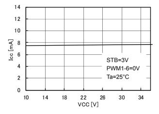
Figure 6. Circuit current
