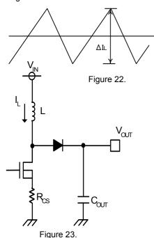
The value of inductor has a great influence on input ripple current. As shown in Equation (1), as the inductor becomes large and switching frequency becomes high, the ripple current of an inductor  $\Delta$ IL becomes low.
