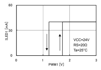
Figure 10. PWM terminal threshold voltage
