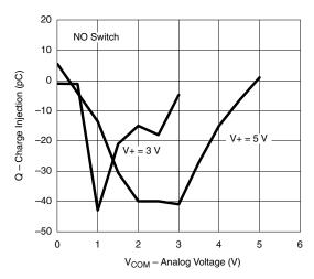
Charge Injection vs. Analog Voltage
