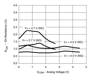
R<sub>ON</sub> vs. V<sub>COM</sub> and Supply Voltage
