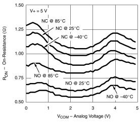
R<sub>ON</sub> vs. Analog Voltage and Temperature
