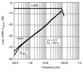
Insertion Loss, Off-Isolation Crosstalk vs. Frequency
