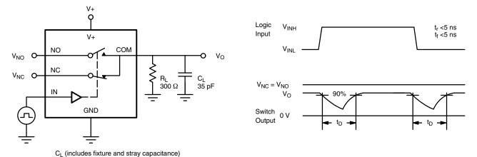
Fig. 2 - Break-Before-Make Interval
