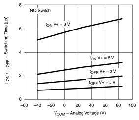
Switching Time vs. Temperature and Supply Voltage
