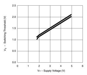
Switching Threshold vs. Supply Voltage
