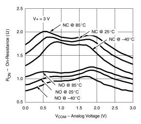
R<sub>ON</sub> vs. Analog Voltage and Temperature
