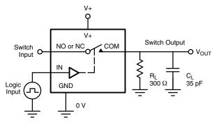
$C_L$  (includes fixture and stray capacitance)
