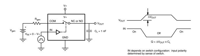
Fig. 3 - Charge Injection
