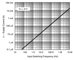
**Supply Current vs. Input Switching Frequency**
