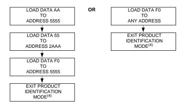
Boot Block Lockout Feature Enable Algorithm<sup>(1)</sup>
