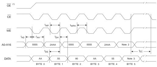
Notes: 1.  $\overline{OE}$  must be high only when  $\overline{WE}$  and  $\overline{CE}$  are both low.
