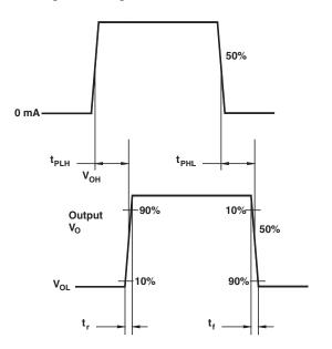
Fig. 10 Switching Times Definition for Inverters
