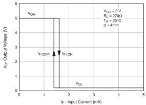
Fig. 2 Output Voltage vs. Input Current (Buffers)
