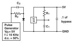
$R_1 = 360\Omega$  $R_2 = 180\Omega$  C<sub>1</sub>= 15 pf C<sub>2</sub>= 20 pf  $C_1$  and  $C_2$  include probe and stray wire capacitance
