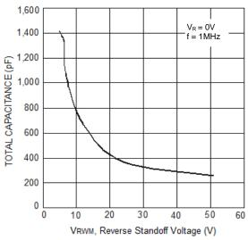
Fig.6 Total Capacitance vs Reverse Standoff Voltage
