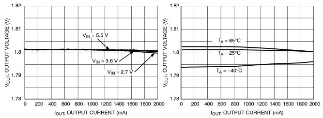
Figure 11. Load Regulation vs. Output Current and Input Voltage (V<sub>OUT</sub> = 1.8 V, T<sub>A</sub> = 25°C)
