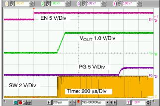
Figure 15. Power Up Sequence and Inrush Current in Input ( $V_{IN}$  = 3.6 V,  $V_{OUT}$  = 1.8 V,  $I_{OUT}$  = 0 A, L = 1.0  $\mu$ H,  $C_{OUT}$  = 10  $\mu$ F)
