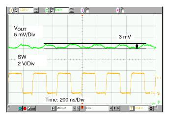
Figure 13. Output Ripple Voltage ( $V_{IN}$  = 3.6 V,  $V_{OUT}$  = 1.8 V,  $I_{OUT}$  = 1 A, L=1.0  $\mu$ H,  $C_{OUT}$  = 10  $\mu$ F)
