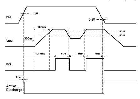
Figure 18. Power Good and Active Discharge Timing Diagram
