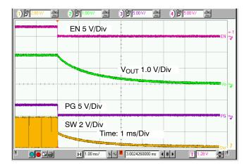
Figure 17. Power Down Sequence and Active Output Discharge ( $V_{IN}$  = 3.6 V,  $V_{OUT}$  = 1.8 V,  $I_{OUT}$  = 0 A, L = 1.0  $\mu$ H,  $C_{OUT}$  = 10  $\mu$ F)
