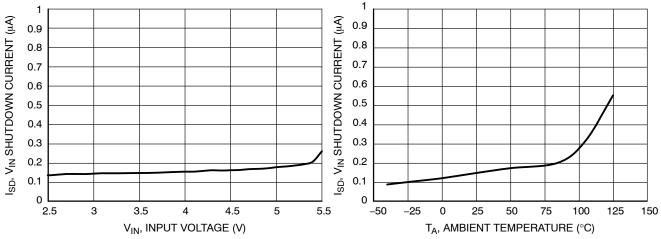
Figure 3. Standby Current vs. Input Voltage (EN = Low,  $T_A = 25$ °C)
