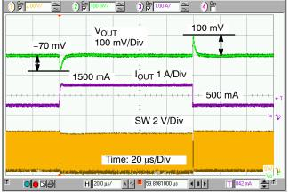
Figure 14. Load Transient Response (V<sub>IN</sub> = 3.6 V, V<sub>OUT</sub> = 1.8 V, I<sub>OUT</sub> = 500 mA to 1500 mA, L = 1.0  $\mu$ H, C<sub>OUT</sub> = 10  $\mu$ F)
