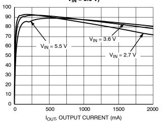
Figure 8. Efficiency vs. Output Current and Input Voltage (V<sub>OUT</sub> = 1.8 V, T<sub>A</sub> = 25°C)
