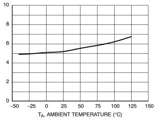
Figure 6. Quiescent Current vs. Temperature (EN = High, Open Loop,  $V_{OUT}$  = 1.8 V,  $V_{IN}$  = 3.6 V)
