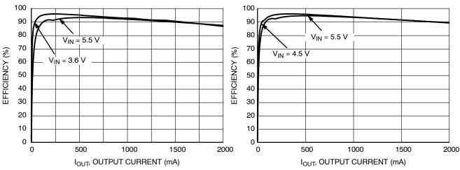
Figure 9. Efficiency vs. Output Current and Input Voltage (V<sub>OUT</sub> = 3.3 V, T<sub>A</sub> = 25°C)
