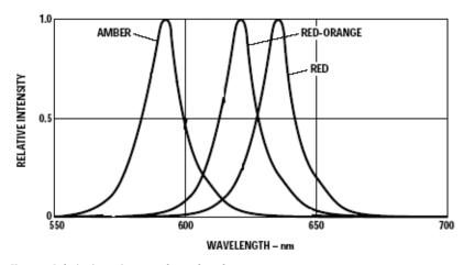
Figure 1. Relative intensity vs. peak wavelength
