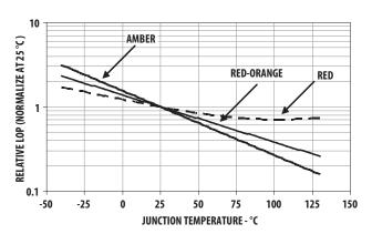
Figure 9. Relative Light Output vs Junction temperature
