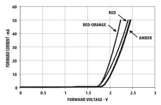
Figure 2. Forward current vs. forward voltage
