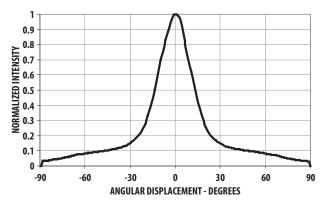
Figure 6. Representative Radiation pattern 30°x70° Lamp -Minor Axis
