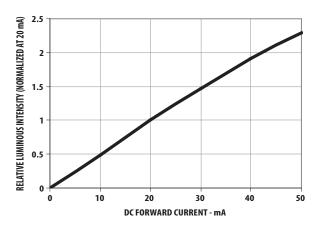
Figure 3. Relative luminous intensity vs. forward current
