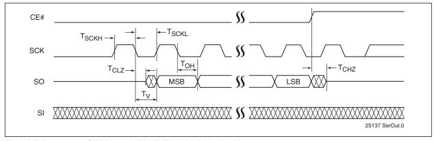
FIGURE 5-2: SERIAL OUTPUT TIMING DIAGRAM
