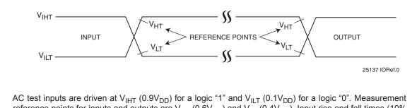
AC test inputs are driven at  $V_{IHT}$  (0.9 $V_{DD}$ ) for a logic "1" and  $V_{ILT}$  (0.1 $V_{DD}$ ) for a logic "0". Measurement reference points for inputs and outputs are  $V_{HT}$  (0.6 $V_{DD}$ ) and  $V_{LT}$  (0.4 $V_{DD}$ ). Input rise and fall times (10%)  $\leftrightarrow$  90%) are <5 ns.
