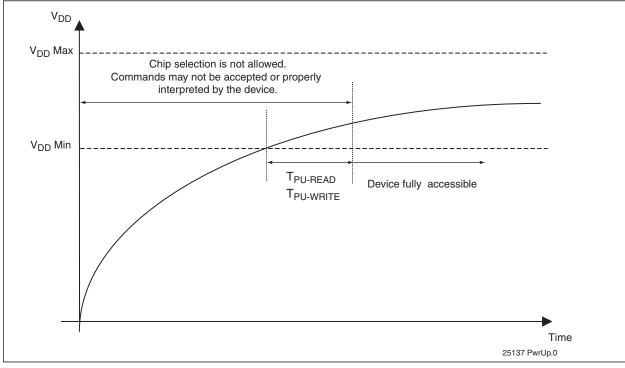
FIGURE 5-4: POWER-UP TIMING DIAGRAM
