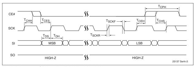
FIGURE 5-1: **SERIAL INPUT TIMING DIAGRAM**
