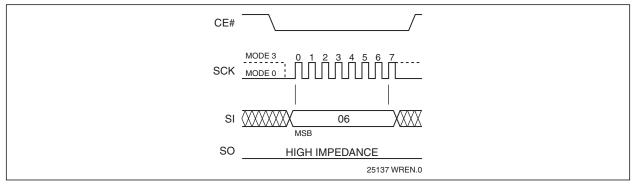
FIGURE 4-15: WRITE ENABLE (WREN) SEQUENCE
