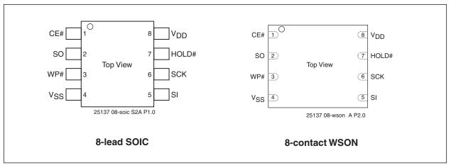
FIGURE 2-1: PIN ASSIGNMENTS
