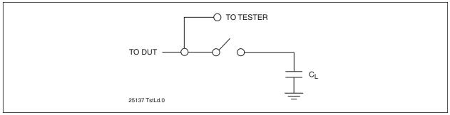
FIGURE 5-6: A TEST LOAD EXAMPLE
