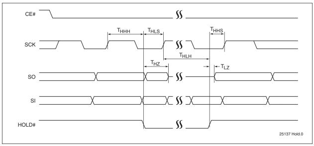
FIGURE 5-3: HOLD TIMING DIAGRAM
