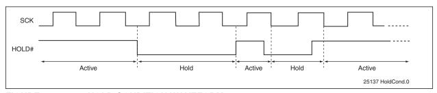
FIGURE 4-2: HOLD CONDITION WAVEFORM
