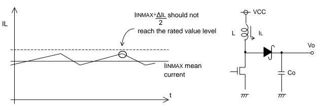
Fig.24 Coil Current Waveform (Step Up DC/DC)
