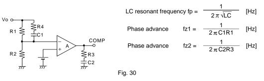
Set a phase advancing frequency close to the LC resonant frequency for the purpose of canceling the LC resonance.
