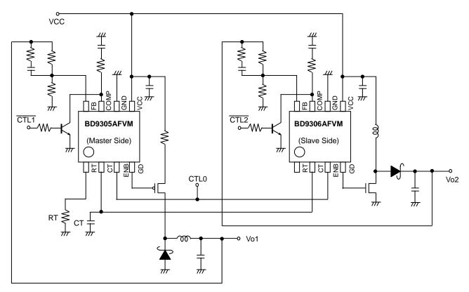
Fig.31 Master Slave Application Circuit
