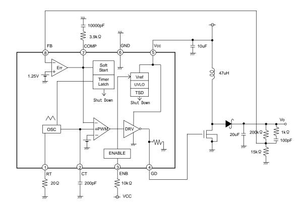
Fig.21 Block Diagram / Application Circuit (BD9306AFVM)
