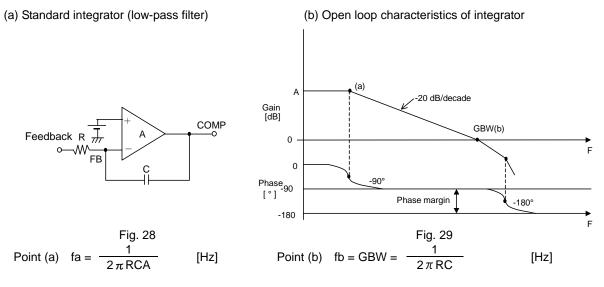
The error amp performs phase compensation of types (a) and (b), making it act as a low-pass filter. For DC/DC converter applications, R refers to feedback resistors connected in parallel. From the LC resonance of output, the number of phase advances to be inserted is two.
