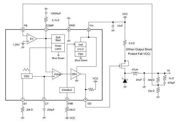
Fig.20 Block Diagram / Application Circuit (BD9305AFVM)
