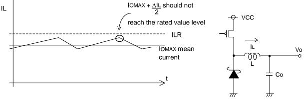
Fig.22 Coil Current Waveform (Step Down DC/DC)
