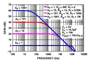
FIGURE 6. FREQUENCY RESPONSE vs CLOSED LOOP GAIN
