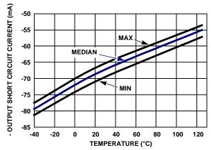
FIGURE 41. - OUTPUT SHORT CIRCUIT CURRENT vs TEMPERATURE  $V_{IN}$  = -2.55V,  $R_L$  = 10,  $V_+$ ,  $V_-$  = ±2.5V
