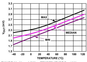
FIGURE 39.  $V_{OUT}$  LOW vs TEMPERATURE R<sub>L</sub>=100k,  $V_+, V_- = \pm 2.5 V$
