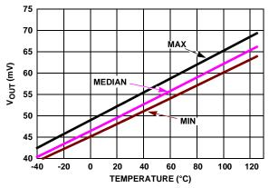
FIGURE 38.  $V_{OUT}$  LOW vs TEMPERATURE  $R_L$  = 1k,  $V_+$ ,  $V_-$  = ±2.5V
