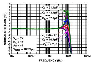
FIGURE 8. GAIN vs FREQUENCY vs CL
