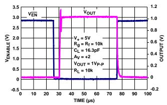
FIGURE 17. ISL28138 ENABLE TO OUTPUT RESPONSE
