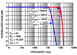
FIGURE 4. GAIN vs FREQUENCY vs  $V_{OUT}$ ,  $R_L = 100k$
