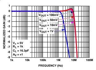
FIGURE 2. GAIN vs FREQUENCY vs V<sub>OUT.</sub> R<sub>L</sub> = 1k
