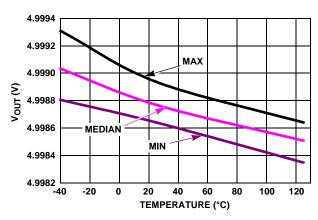
FIGURE 37.  $V_{OUT}$  HIGH vs TEMPERATURE  $R_L = 100k$ ,  $V_+$ ,  $V_- = \pm 2.5V$
