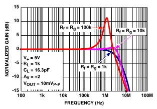
FIGURE 1. GAIN vs FREQUENCY vs FEEDBACK RESISTOR VALUES  $R_{\text{f}}/R_{\alpha}$
