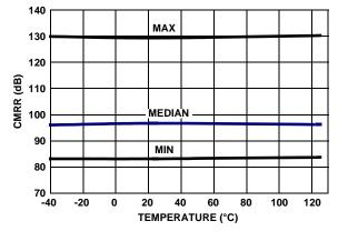
FIGURE 34. CMRR vs TEMPERATURE,  $V_{CM}$  = +2.5V TO -2.5V,  $V_{+}, V_{-}$  = ±2.5V
