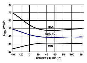
FIGURE 33.  $A_{VOL}$  vs TEMPERATURE,  $R_L$  = 1k  $V_+$ ,  $V_-$  = ±2.5V,  $V_O$  = -2V TO +2V
