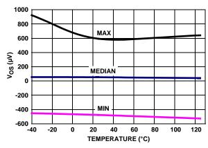
FIGURE 27.  $V_{OS}$  (SOT PKG) vs TEMPERATURE  $V_{IN}$  = 0V,  $V_+$ ,  $V_-$  = ±1.2V
