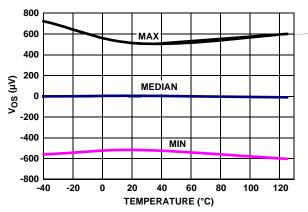
FIGURE 25.  $V_{OS}$  (SOT PKG) vs TEMPERATURE  $V_{IN}$  = 0V, V<sub>+</sub>, V<sub>-</sub> =  $\pm 2.5$ V
