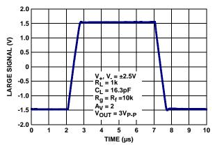
FIGURE 15. LARGE SIGNAL STEP RESPONSE
