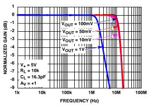
FIGURE 3. GAIN vs FREQUENCY vs V<sub>OUT</sub>, R<sub>L</sub> = 10k
