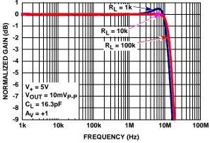
FIGURE 5. GAIN vs FREQUENCY vs RL
