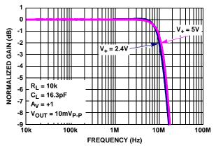
FIGURE 7. GAIN vs FREQUENCY vs SUPPLY VOLTAGE
