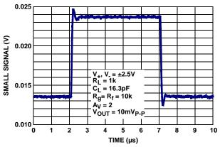
FIGURE 16. SMALL SIGNAL STEP RESPONSE
