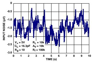
FIGURE 14. INPUT VOLTAGE NOISE 0.1Hz to 10Hz
