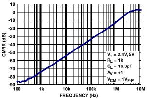
FIGURE 9. CMRR vs FREQUENCY; V<sub>+</sub> = 2.4V AND 5V
