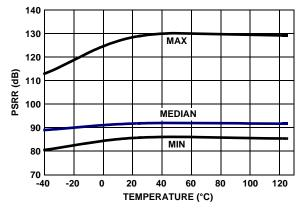
FIGURE 35. PSRR vs TEMPERATURE,  $V_+$ ,  $V_- = \pm 1.2V$  TO
