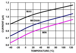
FIGURE 20. SUPPLY CURRENT ENABLED vs TEMPERATURE V<sub>+</sub>, V<sub>-</sub> = ±2.5V
