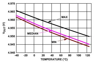
FIGURE 36.  $V_{OUT}$  HIGH vs TEMPERATURE  $R_L$  = 1k,  $V_+$ ,  $V_-$  = ±2.5V
