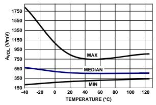
FIGURE 32. A<sub>VOL</sub> vs TEMPERATURE, R<sub>L</sub> = 100k,  $V_+, V_- = \pm 2.5 V, V_O = -2 V TO + 2 V$
