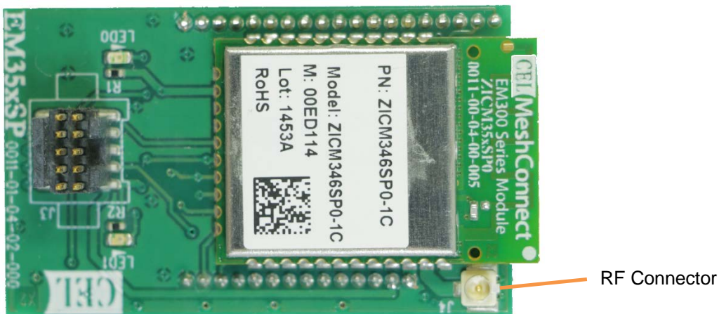
Figure 17. Module with U.FL RF Connector
