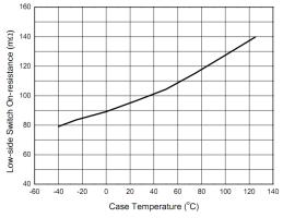
Fig. 6: R<sub>DSONL</sub> versus case temperature
