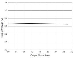
Fig. 9: Output voltage versus output current
