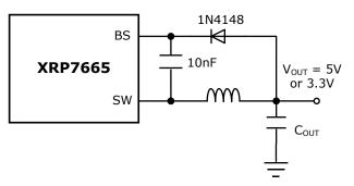
Fig. 17: Optional external bootstrap diode where output voltage is 5V or 3.3V
