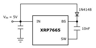
Fig. 16: Optional external bootstrap diode where input voltage is fixed at 5V
