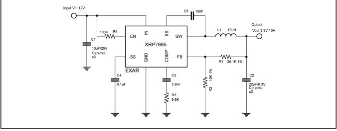
Fig. 1: XRP7665 Application Diagram
