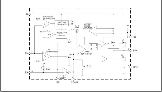
Fig. 2: XRP7665 Block Diagram
