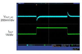
$\label{eq:source} \begin{array}{ll} \mbox{Time} & 200 \mu \mbox{s/div} \\ \mbox{Fig. 11: Load transient (I}_{\mbox{OUT}}\mbox{=}1.5\mbox{A to 3A)} \end{array}$
