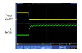
Time 40µs/div Fig. 14: Short-circuit protection
