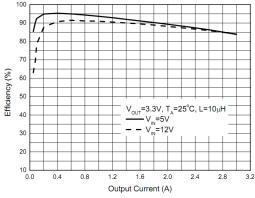
Fig. 4: Efficiency versus output current
