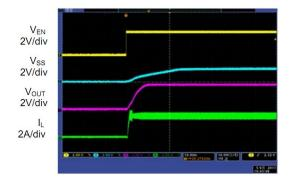
$\begin{array}{rll} \mbox{Time} & 10\mbox{ms/div}\\ \mbox{Fig. 12: Enable turn on}\\ \mbox{CC mode, } V_{IN}\mbox{=}\mbox{12V}, \ V_{OUT}\mbox{=}\mbox{V}_{EN}\mbox{=}\mbox{3.3, } I_{OUT}\mbox{=}\mbox{3A} \end{array}$
