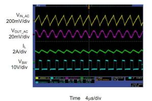
Fig. 10: Output voltage ripple, I<sub>OUT</sub>=3A
