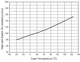
Fig. 5: R<sub>DSONH</sub> versus case temperature
