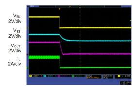
$\label{eq:Fig.13} \begin{array}{l} \mbox{Time} & 200 \mu \mbox{s/div} \\ \mbox{Fig. 13: Enable turn off} \\ \mbox{CC mode, } V_{IN} \mbox{=} 12 \mbox{V}, \mbox{V}_{OUT} \mbox{=} V_{EN} \mbox{=} 3.3, \mbox{ I}_{OUT} \mbox{=} 3A \end{array}$
