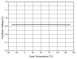
Fig. 7: Feedback voltage versus case temperature
