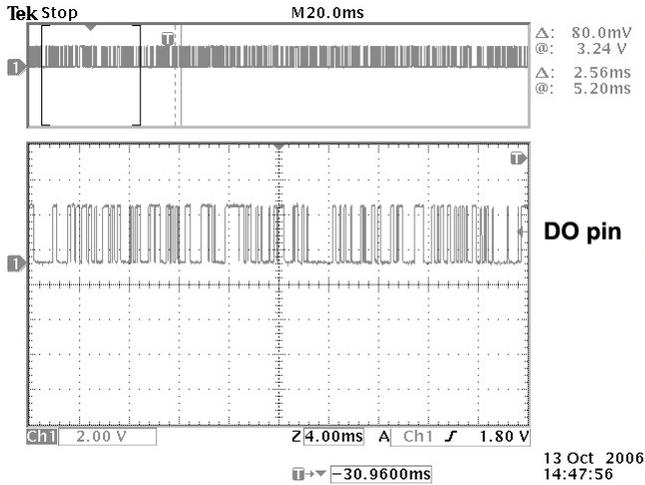
Figure 8. Data Out Pin with No Squelch (SQ = 1).
