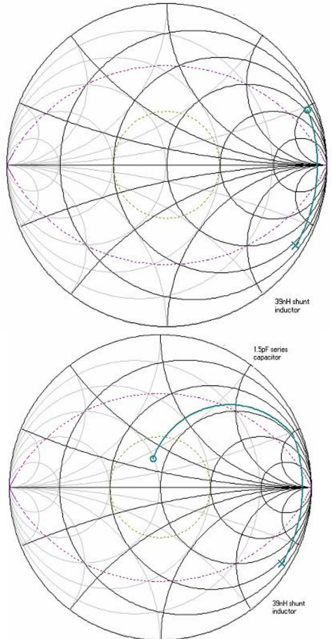
**Figure 5. Plotting the Shunt Inductor and Series Capacitor.**
