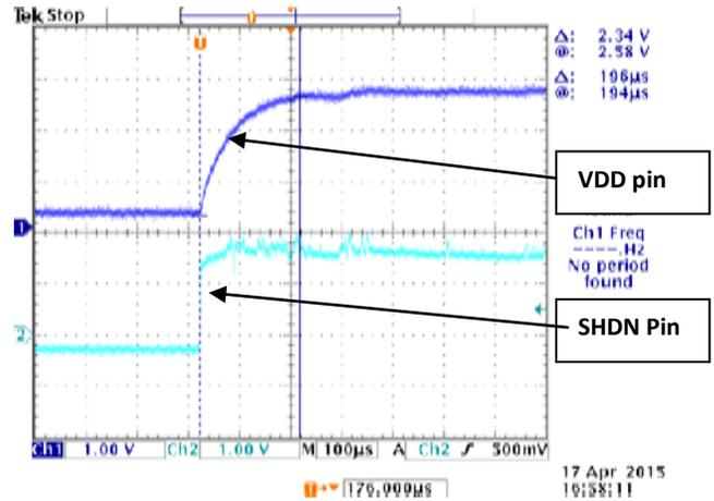
**The suggestion provided above will generally serve to prevent the startup issue from happening to the MICRF211 series ASK receiver. However, exact values of the RC network depend on the ramp rate of the supply voltage, and should be determined on a case-by-case basis.**
