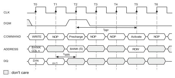
Note: The DQMs can remain low in this example if the length of the write burst is 1 or 2. Write to Precharge
