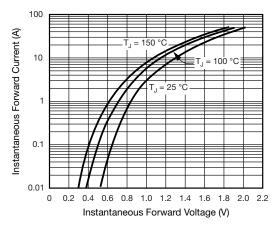
Fig. 4 - Typical Instantaneous Forward Characteristics
