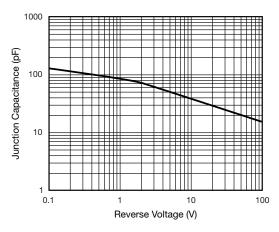
Fig. 5 - Typical Junction Capacitance
