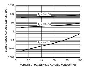
Fig. 3 - Typical Reverse Characteristics
