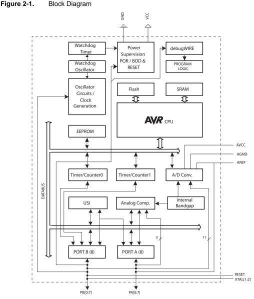
The AVR core combines a rich instruction set with 32 general purpose working registers. All 32 registers are directly connected to the Arithmetic Logic Unit (ALU), allowing two independent registers to be accessed in one single instruction executed in one clock cycle. The resulting architecture is more code efficient while achieving throughputs up to ten times faster than conventional CISC microcontrollers.
