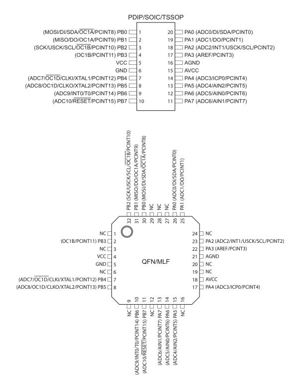
Note: To ensure mechanical stability the center pad underneath the QFN/MLF package should be soldered to ground on the board.
