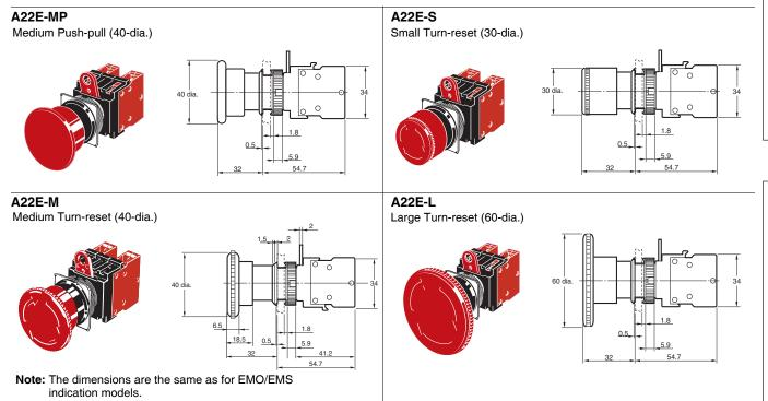
Note: Unless otherwise specified, a tolerance of ±0.8mm applies to all dimensions.
