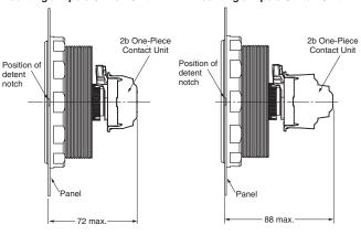
$\boldsymbol{\ast}$  These are the dimension from the front of the panel when the Switch Unit is attached.
