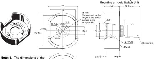
Shroud conform to the specifications of the SEMATECH Application Guide for SEMI S2-93.
