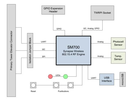
A block diagram for the TWR-RF-SNAP is shown in the figure below.
