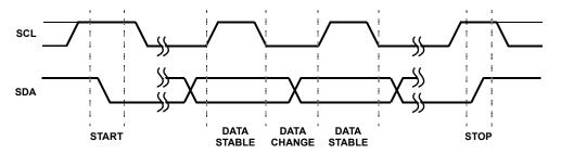
FIGURE 14. VALID DATA CHANGES, START AND STOP CONDITIONS
