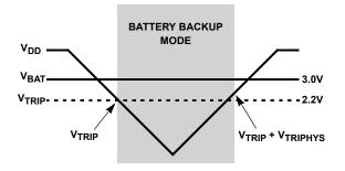
FIGURE 12. BATTERY SWITCHOVER WHEN VBAT > VTRIP
