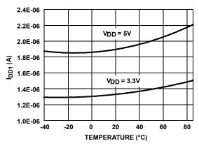
FIGURE 3. I<sub>DD1</sub> vs TEMPERATURE
