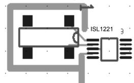
FIGURE 22. SUGGESTED LAYOUT FOR ISL1221 AND **CRYSTAL**
