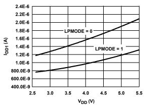
FIGURE 4.  $\rm I_{DD1}$  vs  $\rm V_{DD}$  with LPMode on and off
