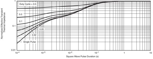
Normalized Thermal Transient Impedance, Junction-to-Case
