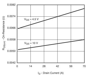
On-Resistance vs. Drain Current and Gate Voltage
