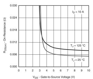
On-Resistance vs. Gate-to-Source Voltage
